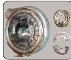
Compressor casing crack
