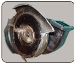
Turbine shell broken
