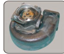
Turbine shell broken
